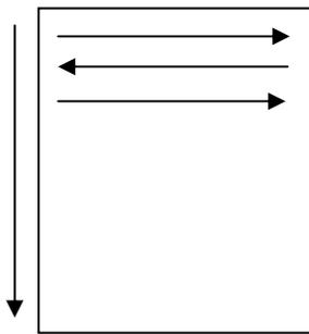
Top-down engraving starts from the top and works its way down.
