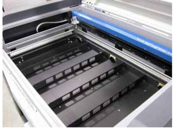
This photo shows the table and supports after the task plate has been removed.
