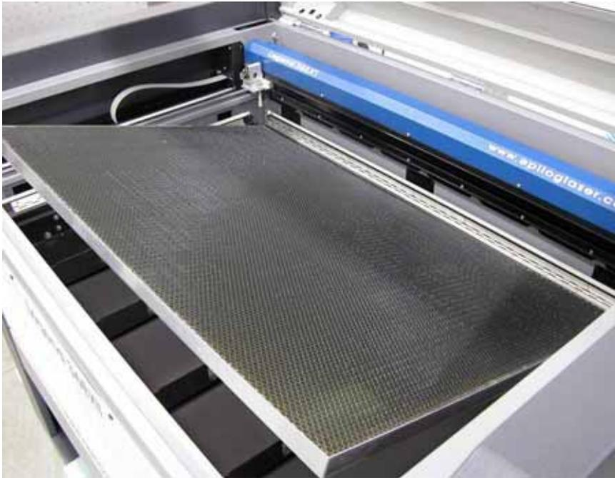
Place the Vector Grid onto the table supports and then flip down the left, right, and top table guides. Your Vector Grid is ready to use.
