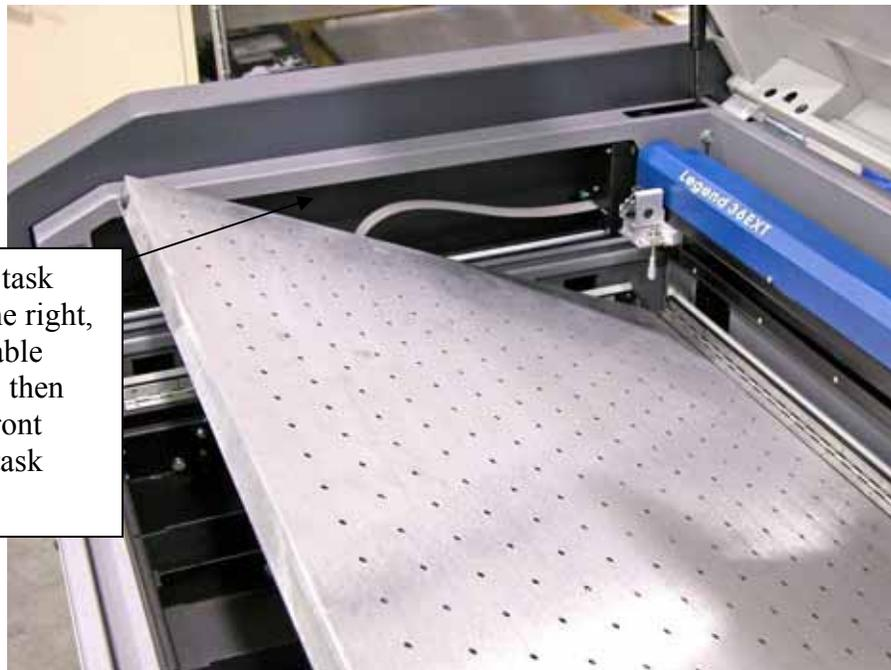
To remove the task plate, flip up the right, left and back table guides (rulers), then lift up on the front corners of the task plate.
