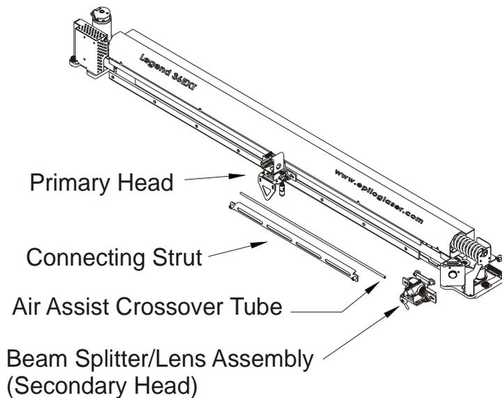
When you are finished using the Double Head, turn the machine off, disconnect the strut, and the air assist crossover tube then remove the beam splitter/lens assembly. “Park” the bearing block at the far right side of the bearing rail.
