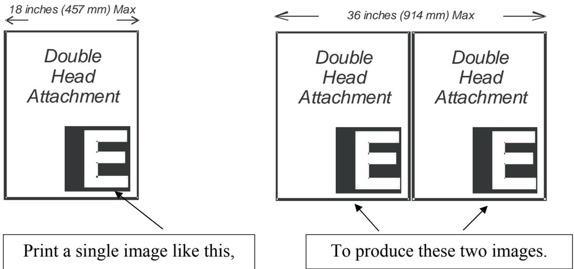
If your system came equipped with the double head attachment the working width of the table in single head mode is reduced from 36 inches (914 mm) to 32 inches (851 mm).
