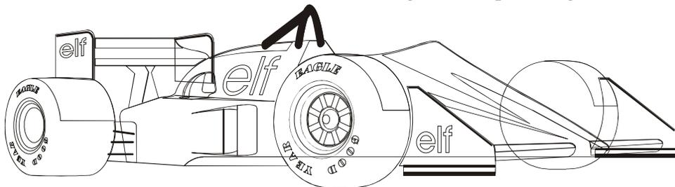
The upper image is a complex piece of clipart. The lower image shows all of the hidden lines that are in this piece of clipart. If this clipart image were run in **Combined mode** it would first raster most of the car then vector cut all but the thickest lines.
