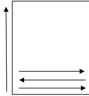
Bottom-Up engraving starts from the bottom and works its way up.
