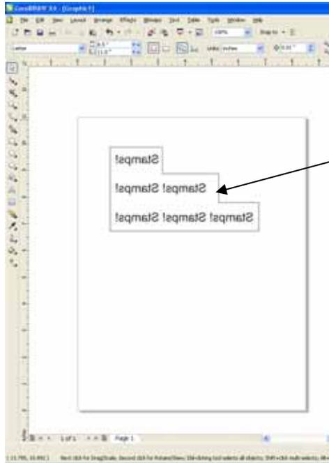
The Fence method uses a *closed outline* to define the area to be engraved away. This image shows the stair-step outline of a Fence enclosing the words to be stamped. The laser will engrave away only the background area outlined by the Fence (leaving the letters standing, of course!).
