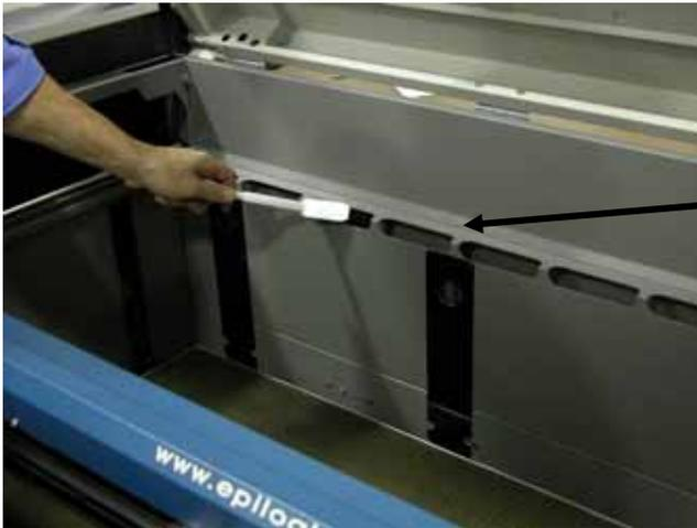
Clean the vents from the inside of the machine. It is best to use a flexible plastic or wire brush that can access the inside of the vent.
