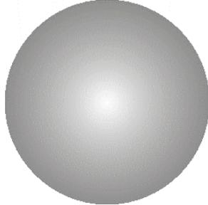
Engraving this circle in 3D mode will create a dome with center being the high point (because it's a light shade of gray) and the outside edge being deep (because it's a darker shade of gray).
