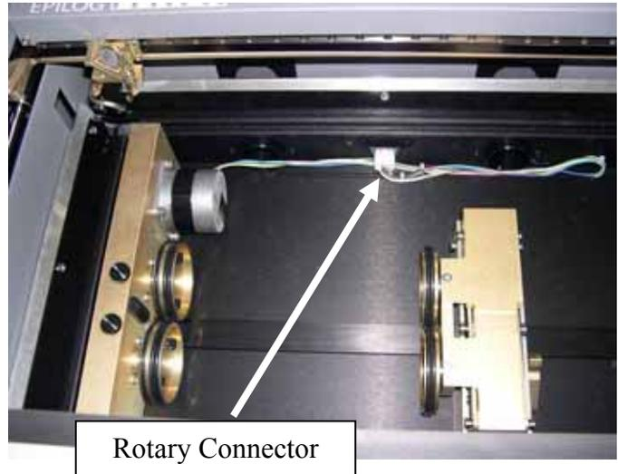
Plug the rotary into the white mating connector located at the rear, center of the Table pan.
