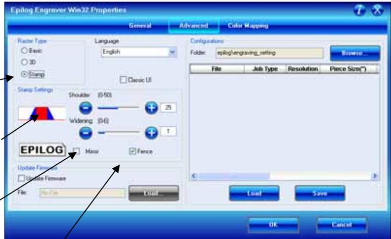
Check the Fence box if necessary.
